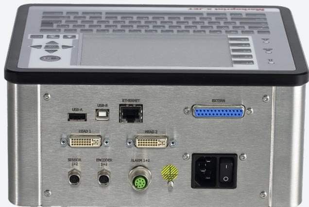
The Markoprint X2JET plus Touch is a 5.7" high-resolution TFT color touchscreen display and controller. The X2JET is used to communicate to a printhead that does not have its own intelligence as well as visualize print jobs and statuses of certain Markoprint printheads that do not have a built-in display. This unit controls a wide array of printheads and head configurations that can adapt to almost any application. It supports four different print technologies: HP, LX, XR & MX Class.
